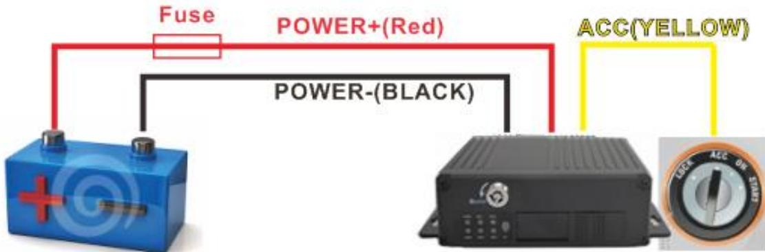
Red Connect Battery(Power) Positive Pole, Black Connect Battery(Power) Negative Pole, Yellow Connect Sole Ignition Switch Or Sole Positive Pole
