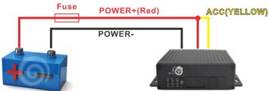
Red and Yellow Together connect Battery(Power) Positive Pole, Black Connect Battery(Power) Negative Pole.
